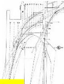
Structures analyzed with **graphic-statics** mathematical calculations, using sectional **drawings to determine compression forces**, bending moments, moments of inertia... (imbalanced lines of compression, destabilize the structure, thrusting outward)
