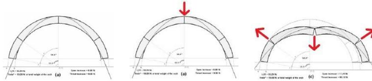
Traditional, **Roman arches** based on **Euclidean geometry**, **circle considered perfect**, resulted in **lateral thrusts**, tending to **collapse if not supported on sides**.
