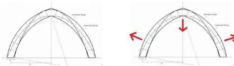
**Gothic arches**, popular in Gaudí's time, base on **two paired circles**, **pointed arch**, also resulted in lateral thrusts, the **lines of compression imbalanced within legs**.
