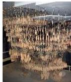
From this plan, hung **system of strings knotted together** representing structural **frame of pillars and arches**, hanging upside down, so **compression loads are inverted into tension**, **pulled by gravity**.
