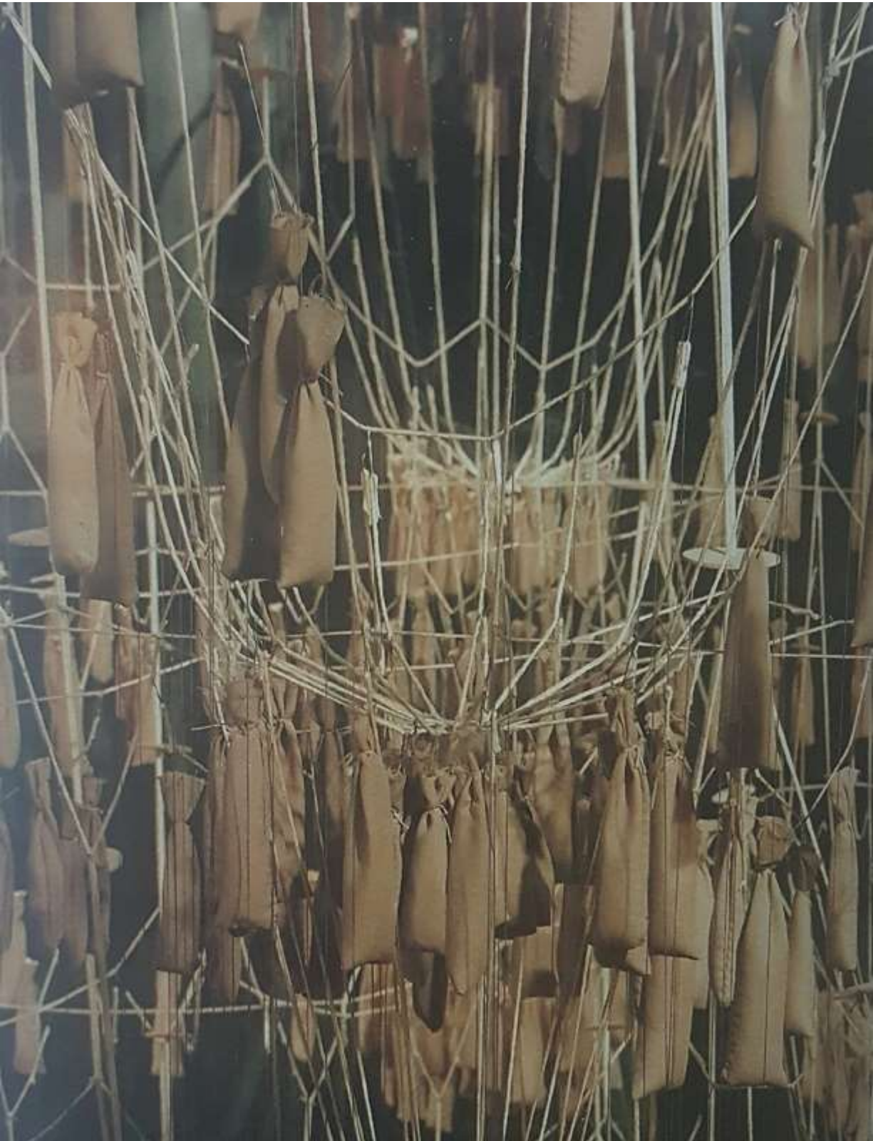
Esterestàtic model by Antoni Gaudí (1898-1908), a system of strings knotted together with weighted bags representing the structural frame of skeletal props and levers, simultaneously and automatically calculating empirically the natural catenary curve of parabolic arches and inclined supports, formed into asymmetric, three-dimensional, dynamic space.
